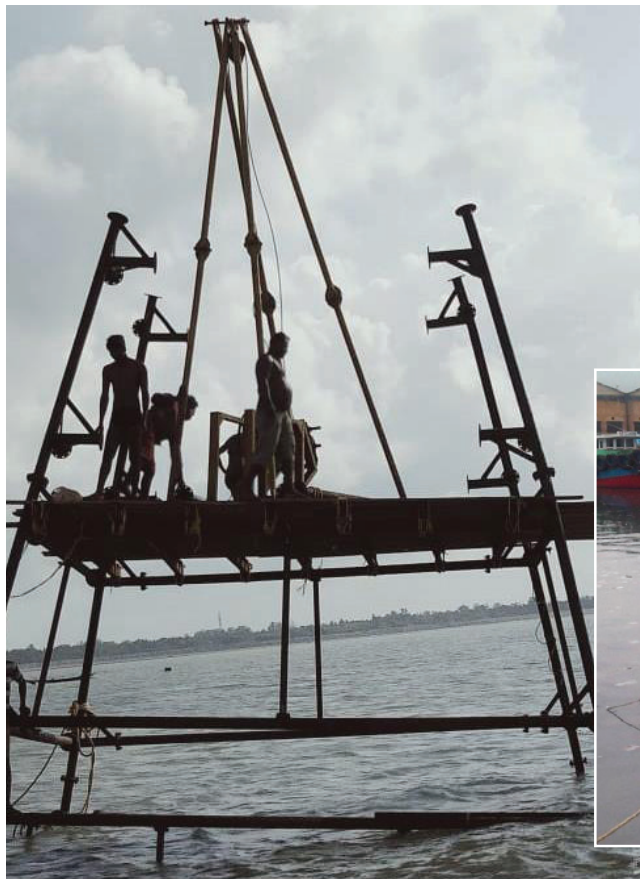
Figure 4-1 and 4-2: Good quality soil investigation cannot be performed with this type of equipment
